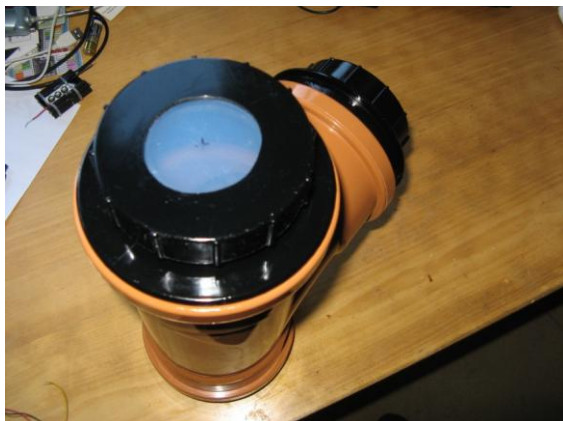
Figure 3.5. The camera window (with the protective masking still in place).
