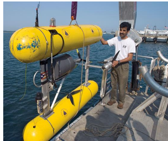
Figure 1.2. SEABED, an autonomous survey vehicle, operated by WHOI [3].
