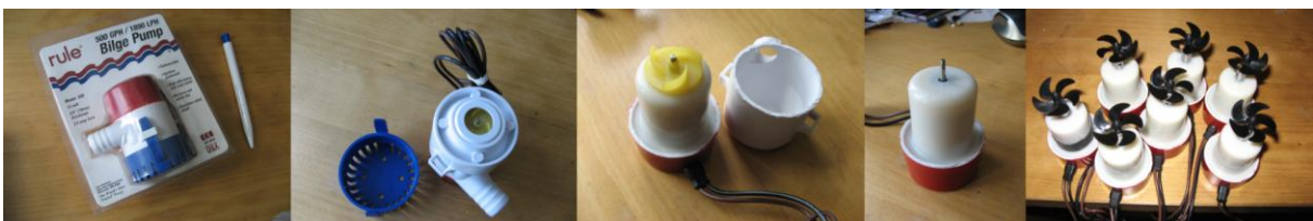
Figure 3.7. Conversion from bilge pump to thruster.
