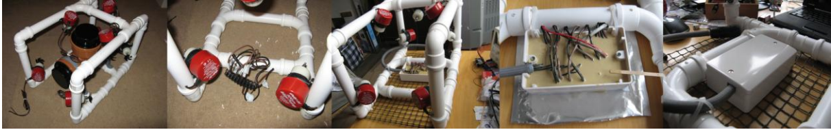
Figure 3.3. Routing and sealing the wiring.
