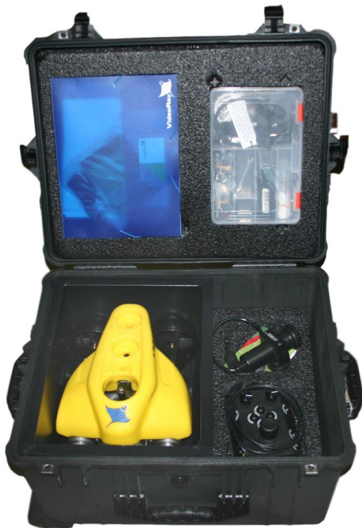
Figure 1.3. The P4 CD 300 is a micro observational class ROV developed by VideoRay LLC [4].
