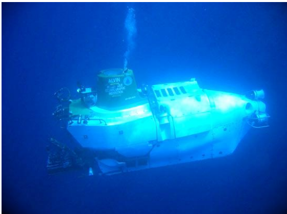
Figure 1.1. ALVIN, a manned underwater vehicle, operated by WHOI [2].
