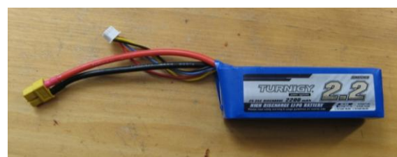
Figure 5.4. Turnigy 2.2 Ah 3S 30C LIPO battery.
