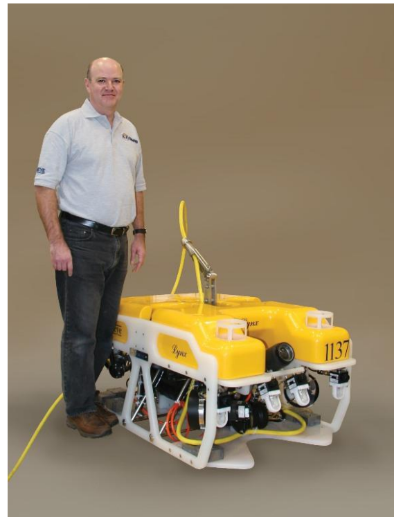
Figure 1.4. The Saab Seacore Lynx is light-medium work class ROV [5].
