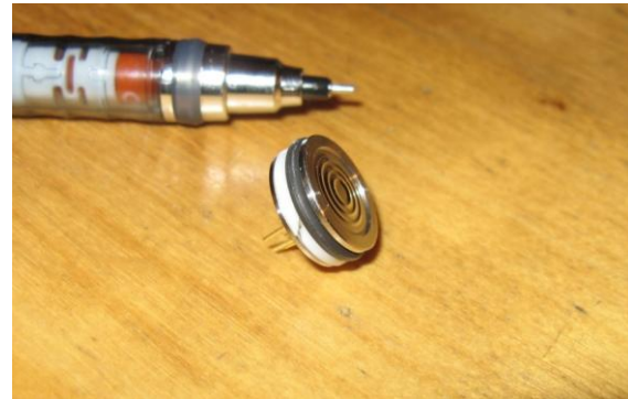
Figure 5.8. Keller PAA-6L pressure transducer.
