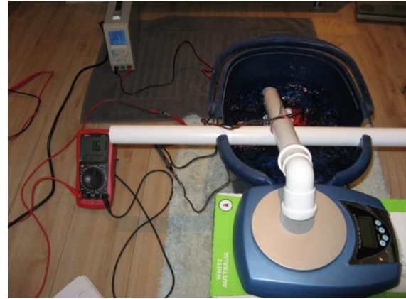
Figure 3.12. Thrust and current draw measurements.
